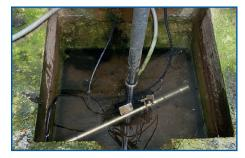
The s::can spectro::lyser industrial is a fully submersible UV/Vis spectrophotometer that measures light absorbance between 190-750nm. s::can's specialized proprietary algorithms analyze & decompose the spectral data to measure for many wastewater parameters: NO<sub>3</sub>-N, COD, CODf & TSS. There are no moving parts in contact with the water & no reagents are used.
