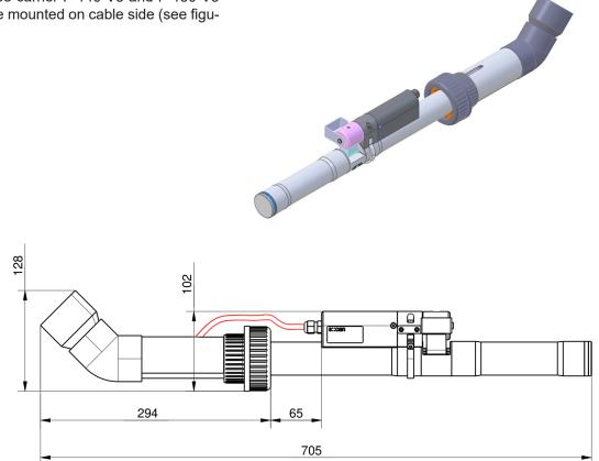
Dimension of probe carrier (F-140-V3) and required space for 35 mm spectrometer with ruck::sack in [mm]
