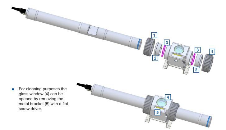
After final mounting the plane face of the measuring section shall have a vertical orientation to avoid any sedimentation in the measuring section and ensure that air bubbles can escape upwards.
