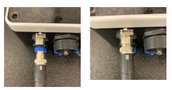
For initialisation on a D-315 con::cube the con::nect B-33-012 must be used. Connect the spectrometer to the con::nect via M12 plug and use a network cable to connect the con::nect to the con::cube. In addition the IP settings of D-315 and spectrometer have to be configured to the same address range (please refer to manual con::nect B-33-012).
