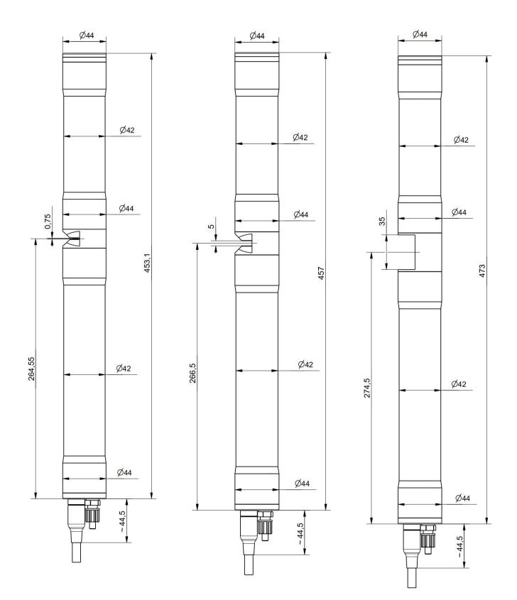
Dimensions of probe in mm:
