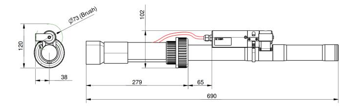
Dimension of probe carrier (F-150-V3) and required space for 35 mm spectrometer with ruck::sack in [mm]
