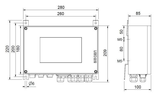
Ensure correct orientation of mounting rails. Top of con::cube has to be tilted backwards to prevent any water flowing over the touch screen or entering the housing when device is opened.
