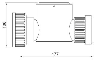
Dimension of flow cell setup in mm (F-48-AMMO)
