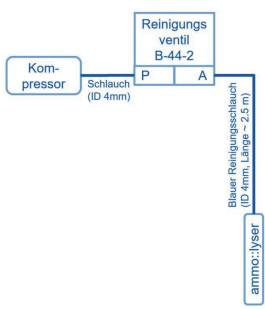
The cleaning valve should never be connected to the compressed air coupling of your compressor directly, i.e. without a pressure hose in between. The total length of hoses should be as short as possible to avoid unnecessary pressure loss. In special occasions, drinking water may be used to operate the hydraulicpneumatic cleaning appliance instead or compressed air.
