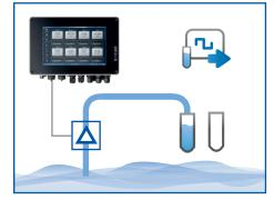
With the con::cube auto-sampler function you can create your own auto-sampler. The conditions for taking samples can be freely configured. It is also possible to combine different conditions and program delays. The sample capacity is controlled either by a fill-level detector or by a timer.
