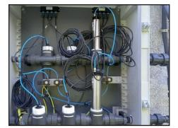
The ammo::lyser is a multi-parameter probe for the online measurement of  $NH_{4}$ ,  $NO_{3}$  and pH. It is an absolutely reliable device outclassing conventional analysers in terms of measurement stability and lifetime. Precision is guaranteed by real-time compensation of the ammonium value with temperature, pH and potassium and a high-performance reference electrode.
