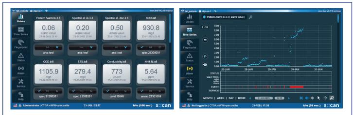
s::can's event detection system continuously analyzes the measured parameters and spectral fingerprint to detect changes in the water composition. Pattern and Spectral alarms can be used to detect deviations from the typical wastewater composition. ana::tool incorporates a simple to use learning system for its alarms that includes user feedback and gradual composition changes (e.g. seasonal variations).
