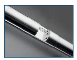
The s::can spectro::lyser™ is a fully submersible UV/Vis spectrophotometer which measures light absorbance between 190 – 750 nm. s::can's proprietary algorithms analyze and decompose the spectral data to provide measurements for many water quality parameters. There are no moving parts in contact with the water and no reagents are used, resulting in almost zero operating costs.
