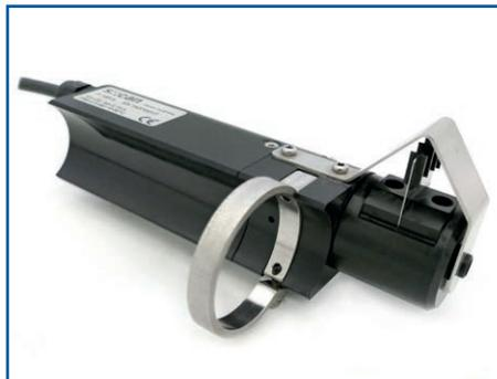
Effective automatic cleaning is a crucial factor when using optical probes in remote locations. The ruck::sack is a submersible rotating brush that reliably removes fouling. With its low power consumption, the ruck::sack is also ideal for battery operation.
