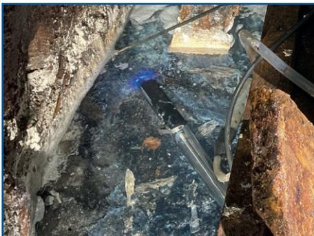
The s::can spectro::lyser™ is a fully submersible UV/Vis spectrophotometer which measures light absorbance between 190 – 750 nm. s::can's proprietary algorithms analyze the spectral data to provide measurements for many water quality parameters. There are no moving parts in contact with the water and no reagents are used, resulting in almost zero operating costs.
