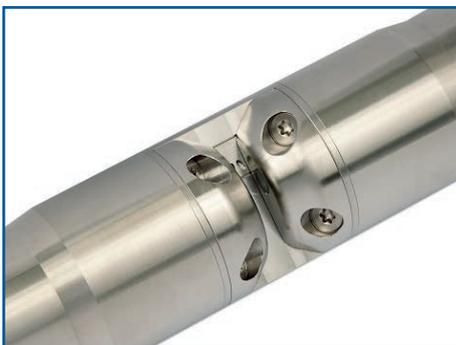
The s::can spectro::lyser industrial is a fully submersible UV/Vis spectrophotometer that measures light absorbance between 190-750nm. s::can's specialized proprietary algorithms analyze & decompose the spectral data to measure for many wastewater parameters: NO<sub>3</sub>N, COD, COD<sub>f</sub> & TSS. There are no moving parts in contact with the water & no reagents are used.
