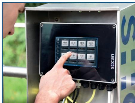
s::can's con::cube is a compact, powerful and versatile terminal for data acquisition and station control. Integrating the newest processor technology, the con::cube has very flexible options for interfacing to SCADA or any central database systems which makes it perfect for station control.
