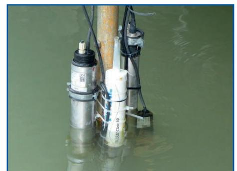
s::can's fully submersible spectro::lyser as well as an ammo::lyser, oxi::lyser and condu::lyser were used to monitor a wide range of parameters all the way from Berlin to the Black Sea. All these sensors require very little maintenance and were ideal for using in multiple applications with long term stability.
