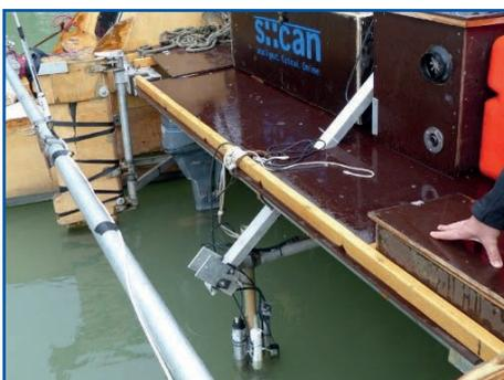
By operating an s::can system on a boat, it is possible to record a nearly complete concentration profile of the organic contaminants (COD, BOD, TOC), nutrients (NH<sub>4</sub>, NO<sub>3</sub>) and the basic parameters pH, temperature, dissolved oxygen and conductivity. Variations in the concentration become visible which allows the tracing of water-polluting discharge points and makes it possible to document them as well as relate them in a way that has never been possible in the past.
