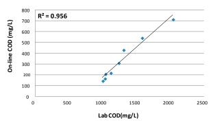
Lab analysis shows, that there is a high correlation between the measurement results from the spectro::lyser and the lab results.
