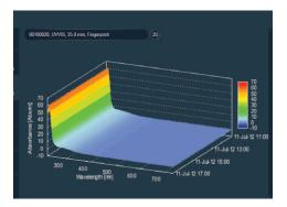
s::can's event detection system continuously analyzes the spectral fingerprint to detect changes in the water composition. The system responds to deviations of parameters compared to the original fingerprint.
