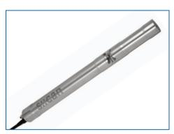
The s::can spectro::lyser™ is a fully submersible UV-Vis spectrometer that measures light absorbance between 190 – 750 nm. s::can's proprietary algorithms analyze and decompose the spectral data to provide measurements for many wastewater parameters including: nitrate, nitrite, COD, BOD, TSS, and dissolved H₂S. There are no moving parts in contact with the water and no reagents are used, resulting in almost no operating costs.
