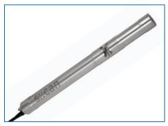
The s::can spectro::lyser™ is a fully submersible UV-Vis spectrometer that measures light absorbance between 190 – 750 nm. s::can's proprietary algorithms analyze and decompose the spectral data to provide measurements for many wastewater parameters including: nitrate, nitrite, COD, BOD, TSS, and dissolved H₂S. There are no moving parts in contact with the water and no reagents are used, resulting in almost no operating costs.
