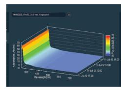
s::can's event detection system continuously analyzes the spectral fingerprint to detect changes in the water composition. The system responds to deviations of parameters compared to the original fingerprint.
