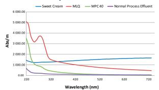
The different dairy products and process effluents have clearly distinguishable spectral fingerprints. This makes a very efficient process control possible resulting in significant cost savings.
