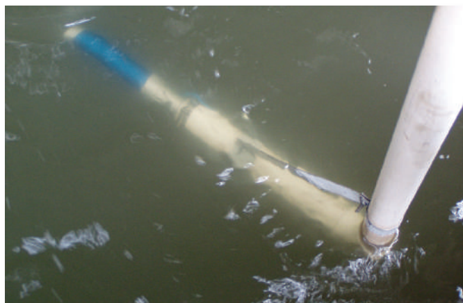
Figure 1. Example of in-situ application of UV-spectroscopy, river water monitoring
