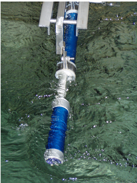
Fig.1: s::can spectrometer probe installed in a spring chamber
