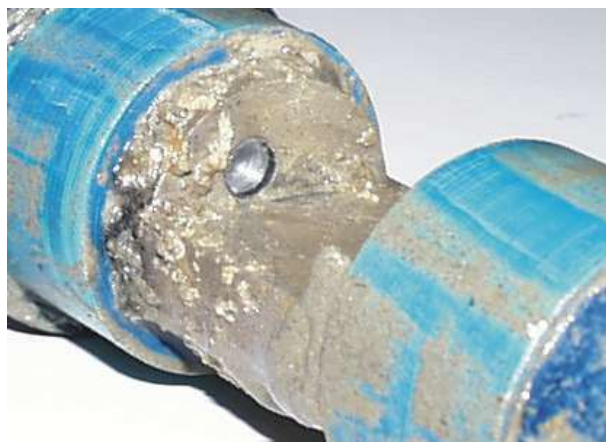
Figure 5: Depositions on the sensor surfaces can lead to deterioration of the sensor signals. Poor long-term stability or high maintenance cost are the consequence. In this case the optical interface has not been affected by the depositions.
