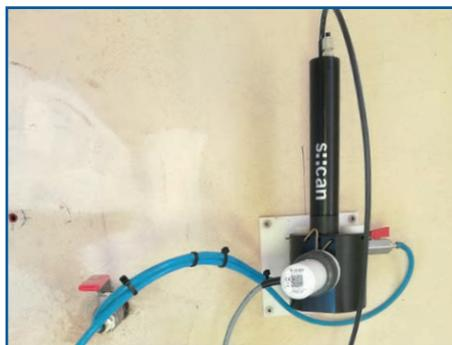
The i::scan is an optical online probe that uses a LED light source and can measure up to eight parameters simultaneously. Parameters that can be measured accurately include Turbidity, TSS, COD, TOC, DOC, Col- or and UV254. Due to the use of multiple wavelengths, cross-sensitivities can be automatically compensated.
