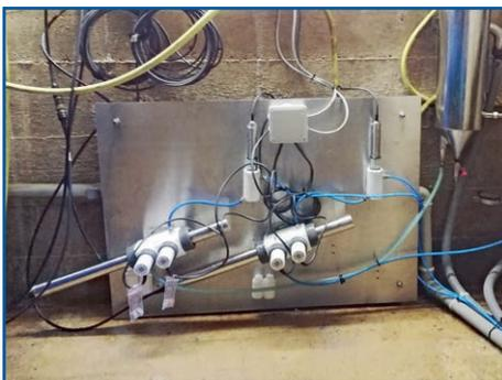
The s::can spectro::lyser™ is a fully submersible UV/Vis spectrophotometer which measures light absorbance between 190 – 750 nm. s::can's proprietary algorithms analyze and decompose the spectral data to provide measurements for many water quality parameters. There are no moving parts in contact with the water and no reagents are used, resulting in almost zero operating costs.
