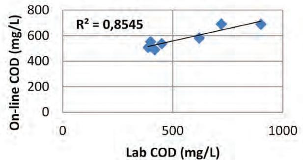
Lab analysis confirms, that there is a high correlation between the measurement results from the spectro::lyser and the laboratory results regarding COD (chemical oxygen demand) in the raw inflow waste water.
