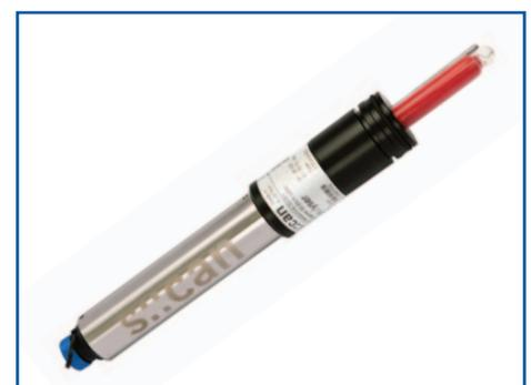
The pH::lyser is a multi-parameter probe that measures the pH value and temperature directly in the water. The pH::lyser uses the temperature to correct the result of the pH measurement online. The non-porous, solid-state reference electrode ensures excellent pH readings and a long lifetime of the electrode especially in harsh environments.
