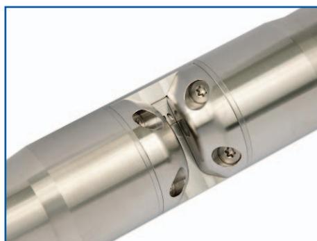
The s::can spectro::lyser™ is a fully submersible UV spectrophotometer which measures light absorbance between 220 – 380 nm. s::can's specialized proprietary algorithms analyze and decompose the spectral data to provide measurements for many important wastewater parameters including: nitrate, nitrite, COD, BOD, TSS, and dissolved H<sub>2</sub>S. There are no moving parts in contact with the water and no reagents are used.
