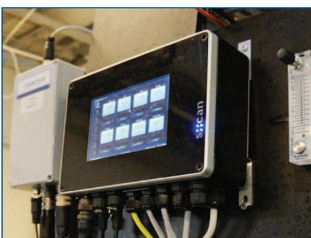
s::can's con::cube is a compact, powerful and versatile terminal for data acquisition and station control. Integrating the newest processor technology, con::cube's very flexible options for interfacing to SCADA or any central database systems makes it perfect for station control. Up to 64 channels/parameters can be displayed.
