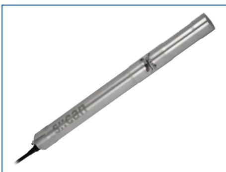
The s::can spectro::lyser™ is a fully submersible UV-Vis spectrometer that measures light absorbance between 190 – 750 nm. s::can's proprietary algorithms analyze and decompose the spectral data to provide measurements for many wastewater parameters including: nitrate, nitrite, COD, BOD, TSS, and dissolved H<sub>2</sub>S. There are no moving parts in contact with the water and no reagents are used, resulting in almost no operating costs.
