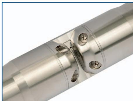
The s::can spectro::lyser industrial is a fully submersible UV/Vis spectrophotometer that measures light absorbance between 190-750 nm. s::can's specialized proprietary algorithms analyze and decompose the spectral data to measurements for many wastewater parameters: NO<sub>3</sub>-N, COD, COD<sub>f</sub> & TSS. Its enhanced specifications make it ideal for industrial applications.
