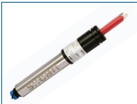
The pH::lyser pro is a multi-parameter probe that measures the pH value and temperature directly in the water. The pH::lyser pro uses the temperature to correct the result of the pH measurement online. The non-porous, solid-state reference electrode ensures excellent pH readings and a long lifetime of the electrode especially in industrial environment.
