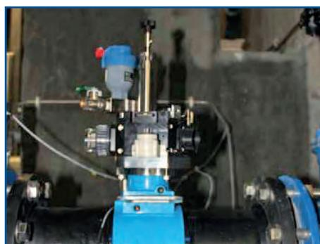
The pipe::scan is a sensor system for monitoring drinking water quality in pipes under pressure. It measures up to 10 parameters in one device: TOC, DOC, UV254, Turbidity, Color, Chlorine, pH/Redox, Conductivity, Temperature and Pressure. The water quality data can be sent to any central database via almost any protocol. Multiple pipe::scans are the ideal solution to monitor drinking water at any point in the network.
