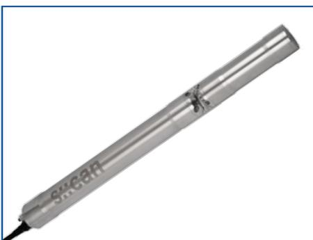
The s::can spectro::lyser™ is a fully submersible UV-Vis spectrometer that measures light absorbance between 220 – 720 nm. s::can's proprietary algorithms analyze and decompose the spectral data to provide measurements for many wastewater parameters including: nitrate, nitrite, COD, BOD, TSS, and dissolved H<sub>2</sub>S. There are no moving parts in contact with the water and no reagents are used, resulting in almost no operating costs.
