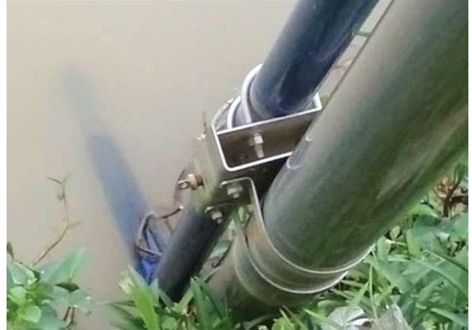
Figure 1: River water monitoring using the s::can spectro::lyser™
