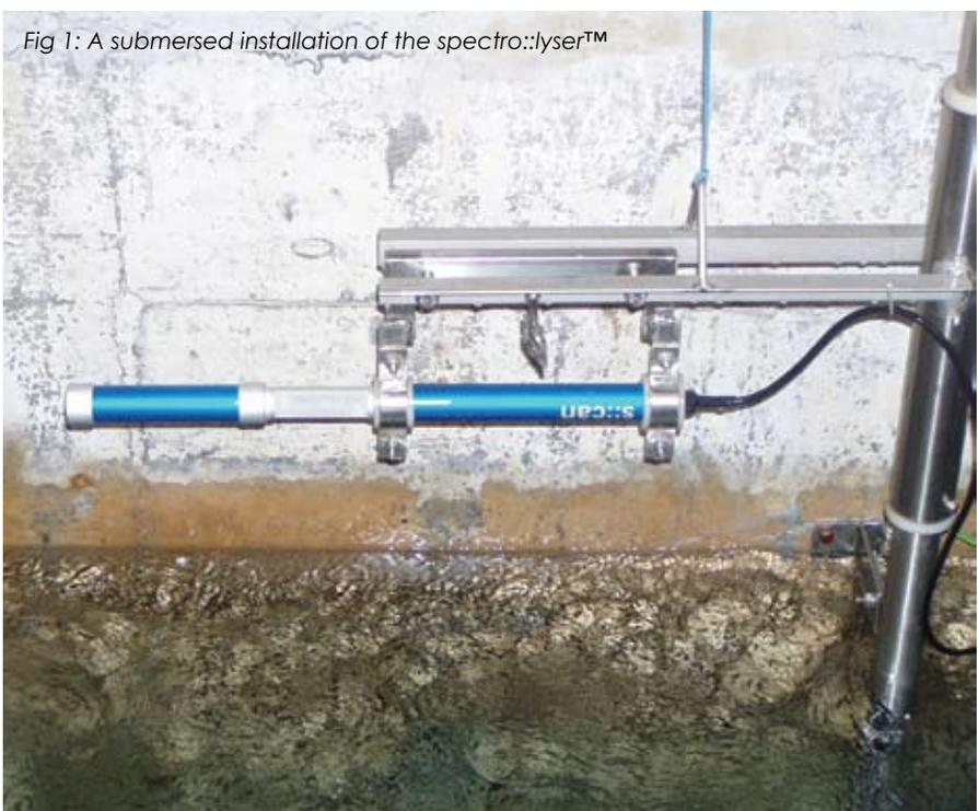
Fig 1: A submersed installation of the spectro::lyser™
