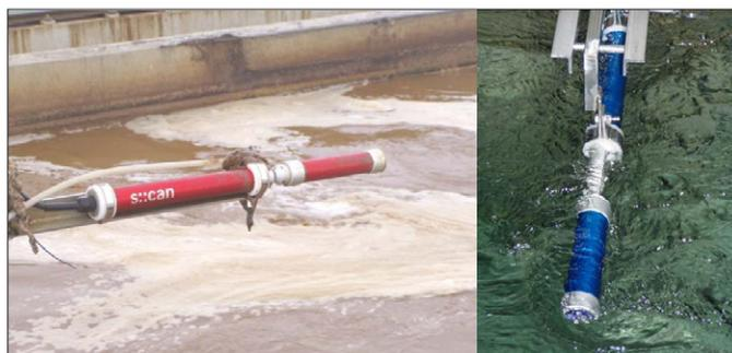
**Figure 1.** Examples of *in situ* applications of UV spectroscopy; process control in a wastewater treatment plant (left) and drinking water monitoring (right).
