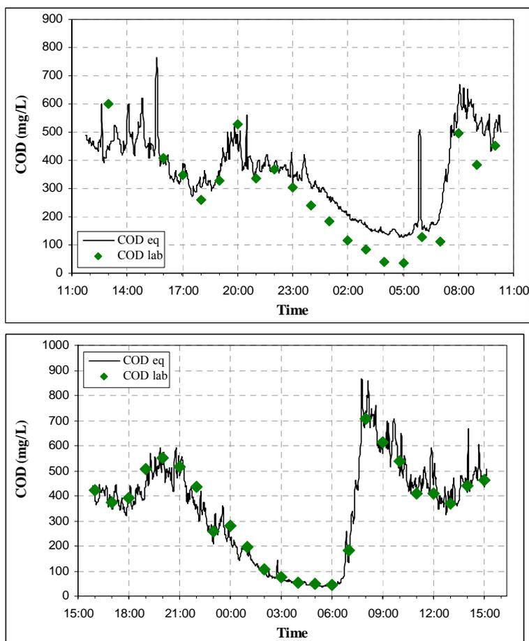
**Figure 5** Best possible “on-line” calibration in July 2004 (top) and adapted “off-line” local calibration in September 2004 (bottom), both during dry weather in Ecully.
