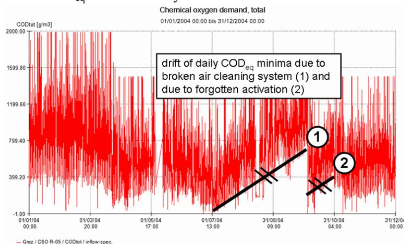
**Figure 7** (1): Same drift of daily CODEq minima due to a broken air cleaning system and (2) due to a forgotten activation of the compressor of the air cleaning system
