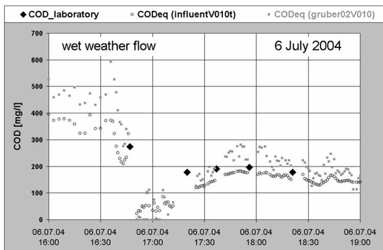
**Figure 6** Comparison between the global calibration of the manufacturer (influentV010t), a new local calibration (gruber02V010) and spot lab samples during wet weather condition in Graz
