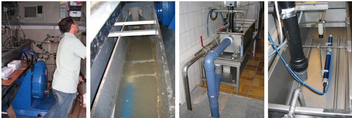
**Figure 2** Bypass installations in Ecully with a peristaltic pump (two left photos) and in Vienna with a submersible shredding pump (two right photos) for wastewater supply to measurement flumes containing the sensors
