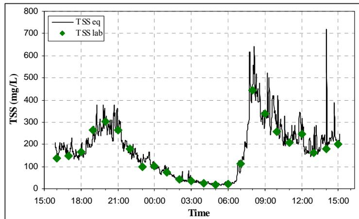
**Figure 3** Equivalent TSS concentration and laboratory TSS concentration after local calibration in Ecully (dry weather 24h period in July 2004).
