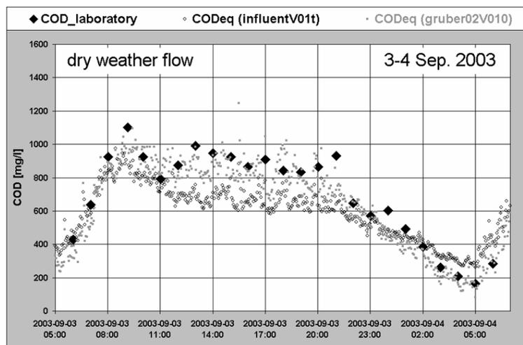
**Figure 4** Comparison between the global calibration of the manufacturer (influentV01t) and a new calibration set locally adjusted to the wastewater matrix in Graz (gruber02V010) for COD
