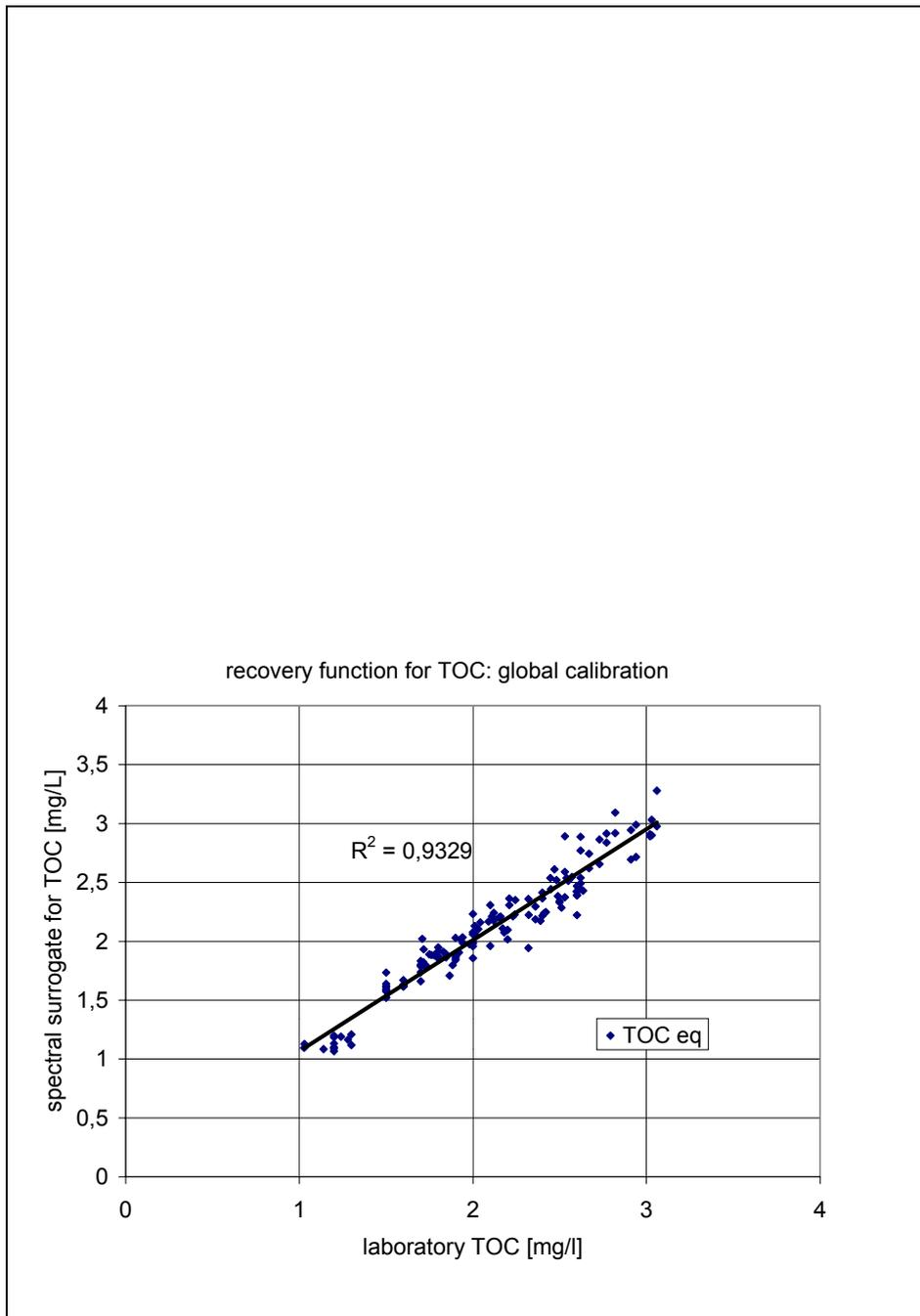
Figure 5: Recovery function for TOC and spectral measurement of a surrogate parameter.
