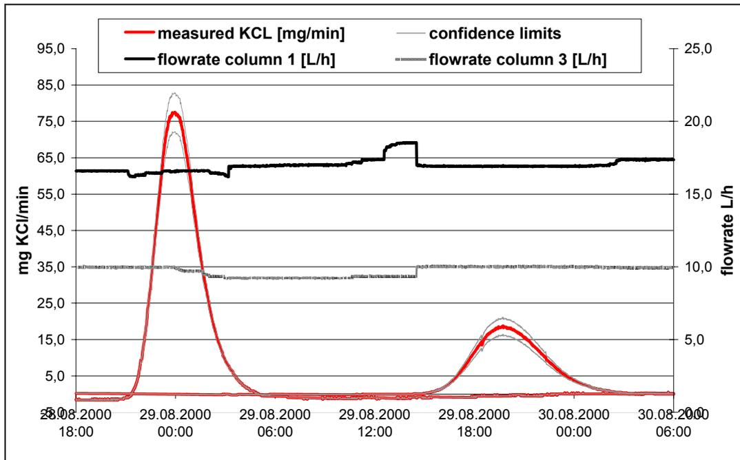
Figure 1: Results of one tracer experiment with 17L/h in the first column and 10 L/h for the third column (right ordinate). The strong line with two peaks shows the KCl load in mg/min (left ordinate) and the respective confidence limits.
