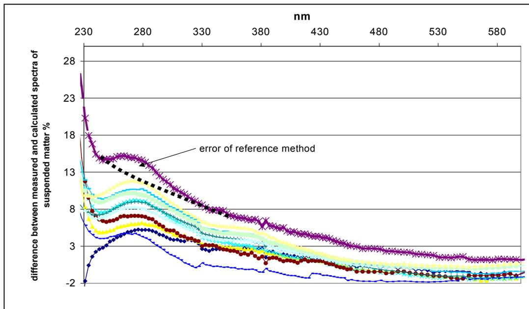
Figure 4: Difference between measured and calculated spectra of suspended matter. The shoulder in the wavelength region between 250 nm – 340 nm is due to errors induced by the filtration process itself. Theoretically spectra of suspended matter do not show any spectral shape but exponential increase with shorter wavelengths.
