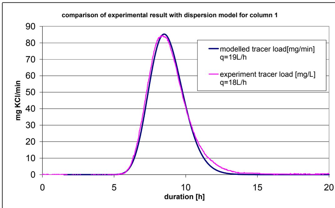
Figure 2: Comparison of measured tracer load in column 1 with calculations from a simple dispersion model fitted to the experimental data.
