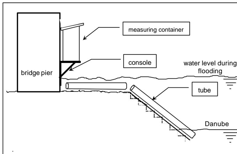
Figure 2: Principle layout of the Danube river monitoring station
