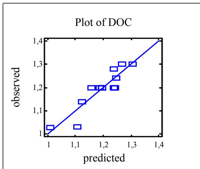
Figure 5. Calibration of the “spectro::lyser” using only bank filtration measurements.
