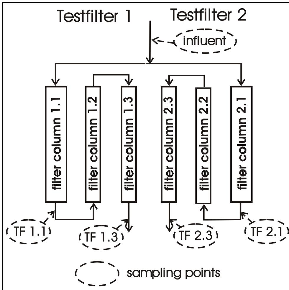
Figure 1. Scheme of the testfilter.
