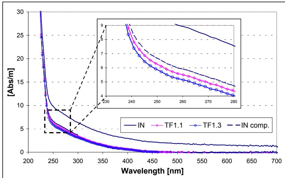
Figure 3. UV/VIS fingerprints for Testfilter 1 (IN ... influent, TF1.1 ... TF1 effluent column 1, TF1.3 ... TF1 effluent column 3, IN ... turbidity compensated influent).
