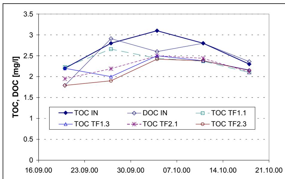
Figure 2. TOC measurements (IN ... influent, TF1.1 ... TF1 effluent column 1, TF1.3 ... TF1 effluent column 3, TF2.1 ... TF2 effluent column 1, TF2.3 ... TF2 effluent column 3).
