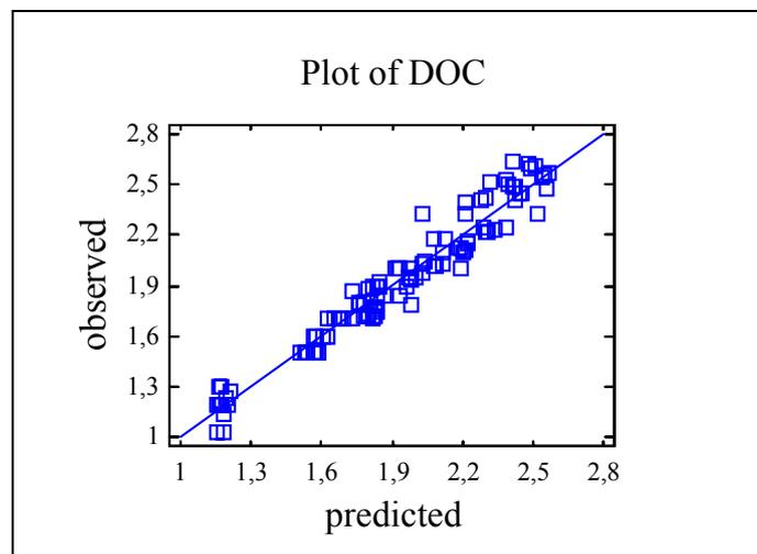
Figure 4. Calibration of the “spectro::lyser” using all testfilter and bank filtration data ( $r^2=95\%$ , mean error = 0.07 mg/l).
