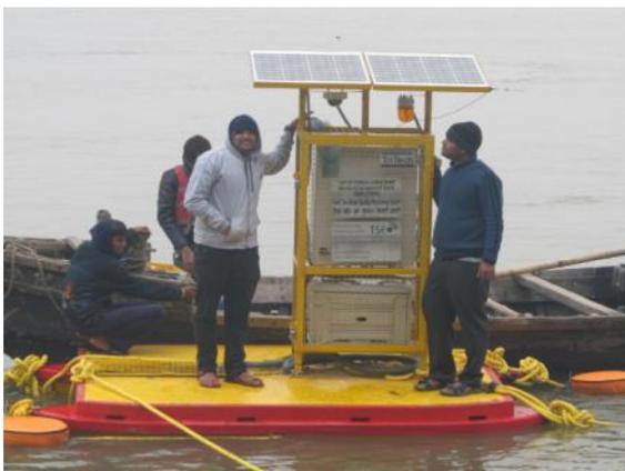
Figure 1.2. Floating monitoring station
