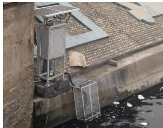
Figure 1.3. River side monitoring station
